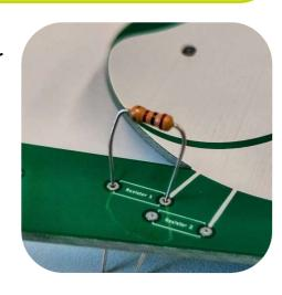
Flip the board over and bend the legs gently so that the resistor doesn't fall out.
